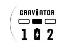
Your Graviator is fully charged when the LED 1 and 2 lights green and the charging indicator is turned off.
