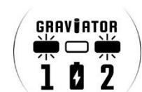
After pressing the button. LED 1 and 2 flashes alternately green until there is made connection with the server.
